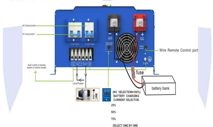
Battery charging current: battery charging current selector on 100% (100% is the maximum Battery charging current) and the selection of the s
